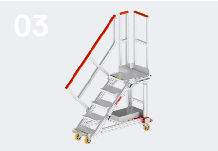
Example with a special version width of 450 mm and aluminium grooved R11; 45°; handrail on both sides; counterweight
