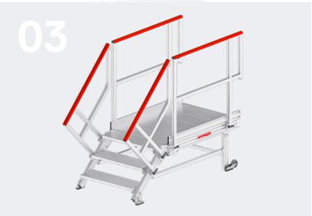
Example with a special version width of 800 mm and aluminium grooved R11; 45°; handrail on both sides; overhang
